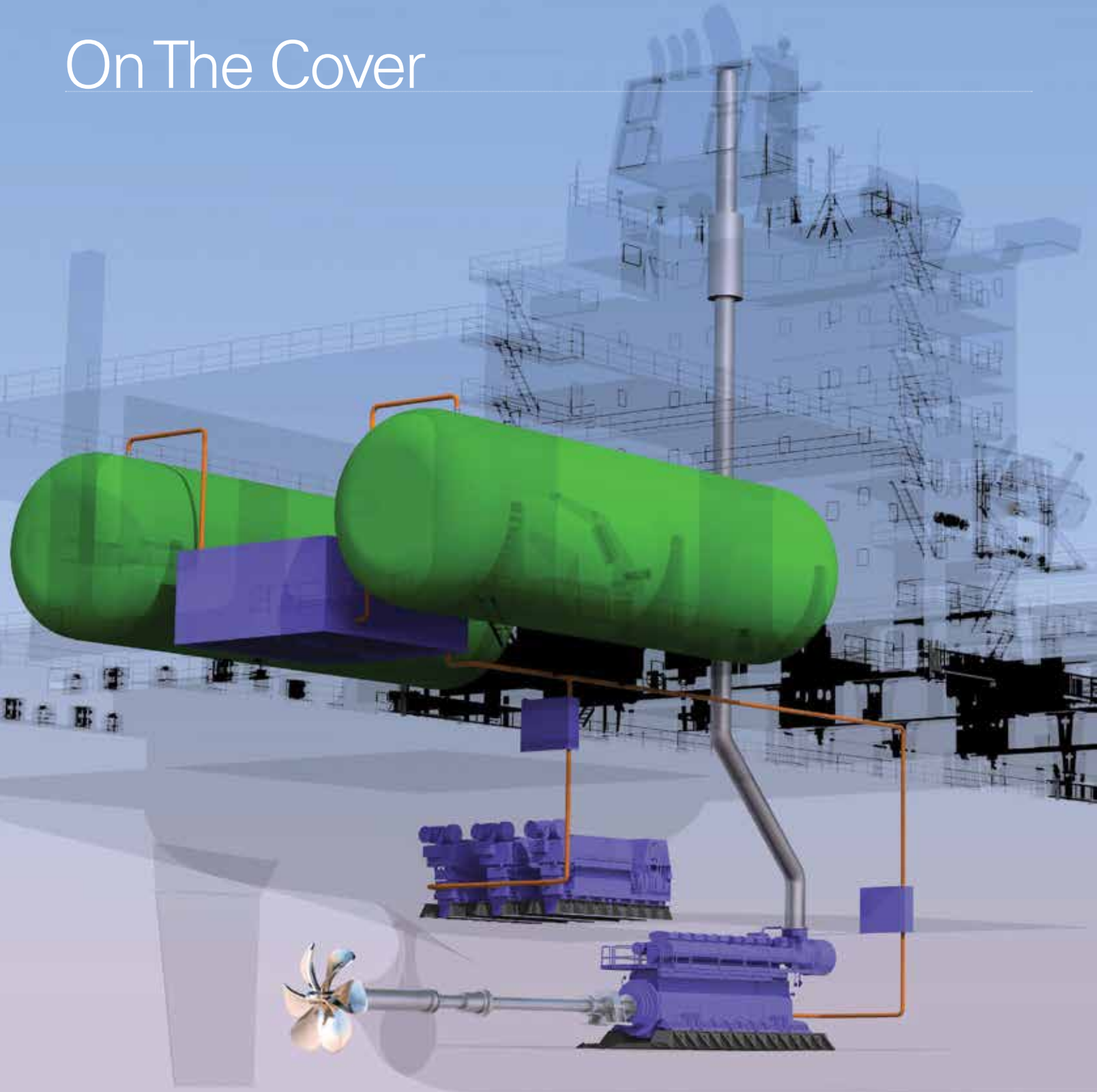
Artist's rendering of the LNG fuel system for TOTE Maritime's LNG-powered container ships.
