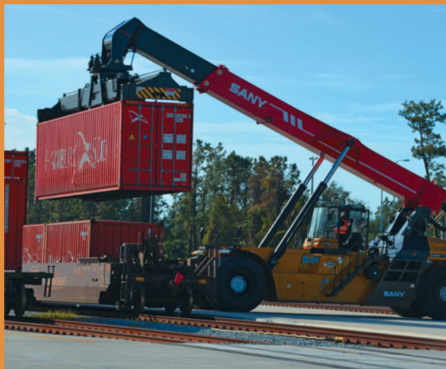
SANY’s super-duty reach stacker efficiently moves containers between rail and truck with a 50-ton, second-rail lift capacity.
