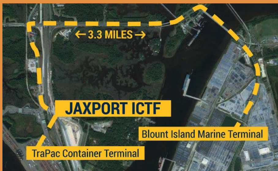
The ICTF allows cargo to move quickly between rail and the adjacent seaport terminal docks, slashing drayage from 20 miles to three miles or less.
