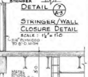
STRINGER/WALL CLOSURE DETAIL SCALE: 1/2" = 1'-0"
