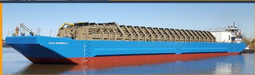
TOTE Maritime is launching North America's first LNG bunker barge, Clean Jacksonville, for barge-to-ship LNG bunkering.
