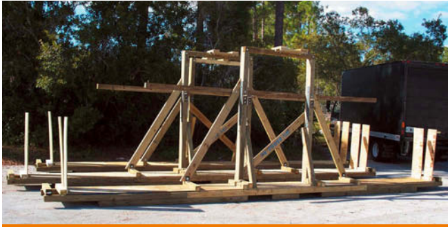
Specialized packing crate for a motorcycle or other unique item built to fit securely inside a shipping container.
