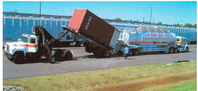
Bulkmatic's innovative transfer technique for moving dry bulk from container to trailer or rail car.
