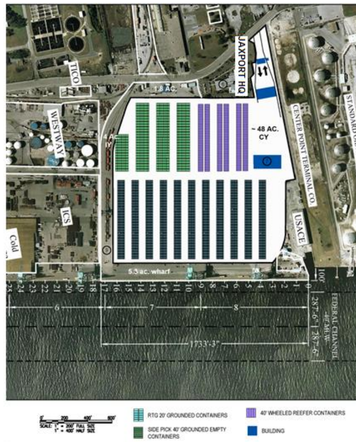
Exhibit V-18 - Conceptual Layout of a Shallow Draft Container Terminal at Talleyrand Marine Terminal
