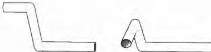
Figure 3-4: Inlet when using 2 and/or 3 dimensional bends upstream of the flowmeter
