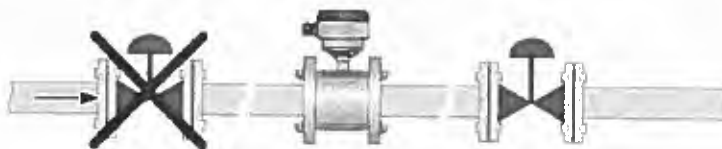
Figure 3-11: Installation in front of a control valve
