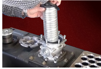
Spin-on Breather, Wire Mesh Strainer & Replaceable Internal Element (Standard)
