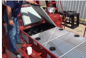
Lightweight Deck Lids and Easy Access to Heavy Duty Circuit Breaker Panel
